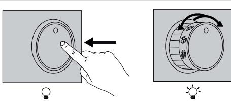
**Lights** - To turn the lights on, press the dial and release it so that it pops out of its housing. To turn the lights off, push the dial back inwards, returning it to the off position.
